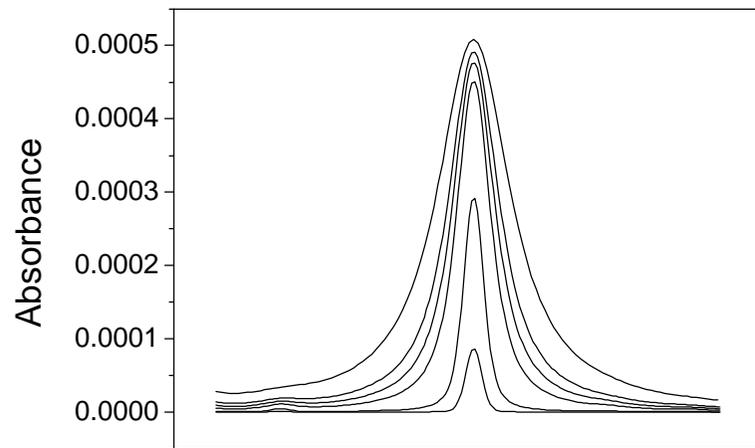
Analytical H<sub>2</sub>O spectral line shapes for different NH<sub>3</sub> pressures: 760, 500, 400, 300, 100, 20 Torr.
