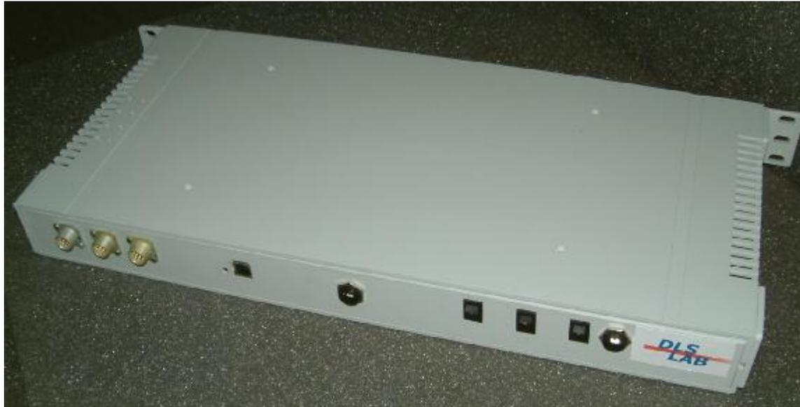
View of 3 channels TDLS complex developed to measure NH<sub>3</sub> in AsH<sub>3</sub> and PH<sub>3</sub>.
