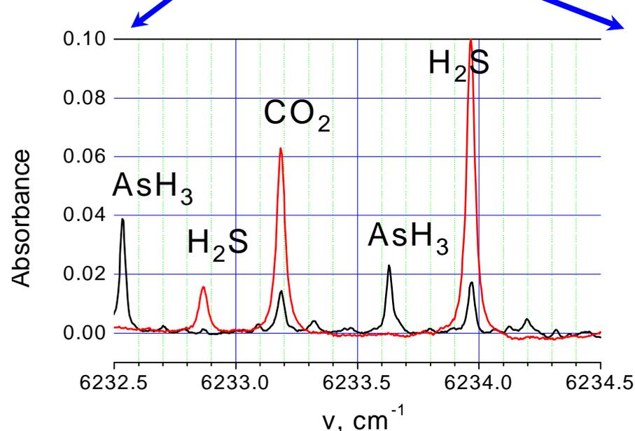
Analytical lines to detect CO<sub>2</sub> and H<sub>2</sub>S were selected to have no interference with AsH<sub>3</sub> absorption.
