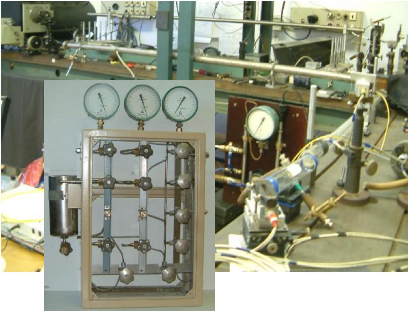
View of 3 channels DL based spectrometer developed with gas distribution system to deal with hazard objects.
