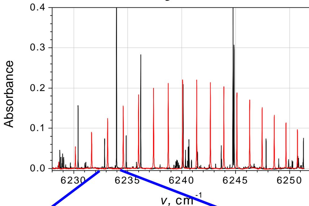
Absorption spectra of CO<sub>2</sub> (red) and H<sub>2</sub>S (black) in spectral range under consideration as recorded by TDLS.
